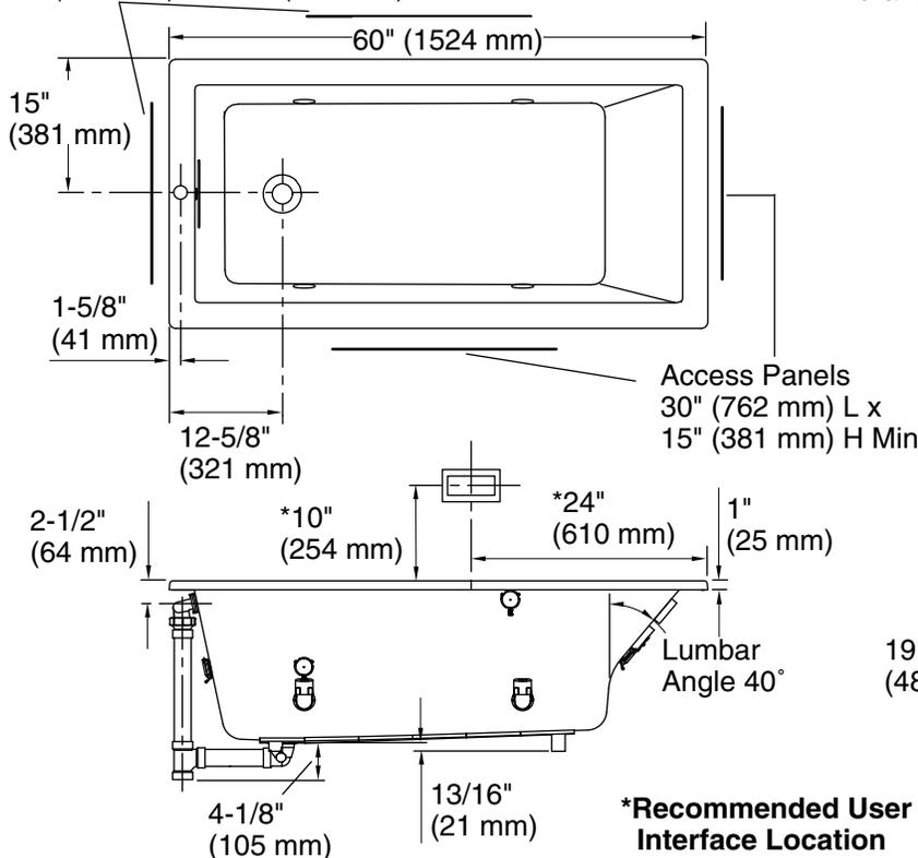
No change in measurement if connected with drain illustrated. (K-7272)
